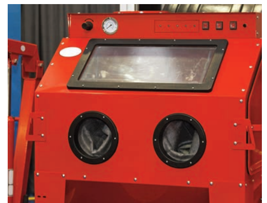
Enclosure for sandblasting
